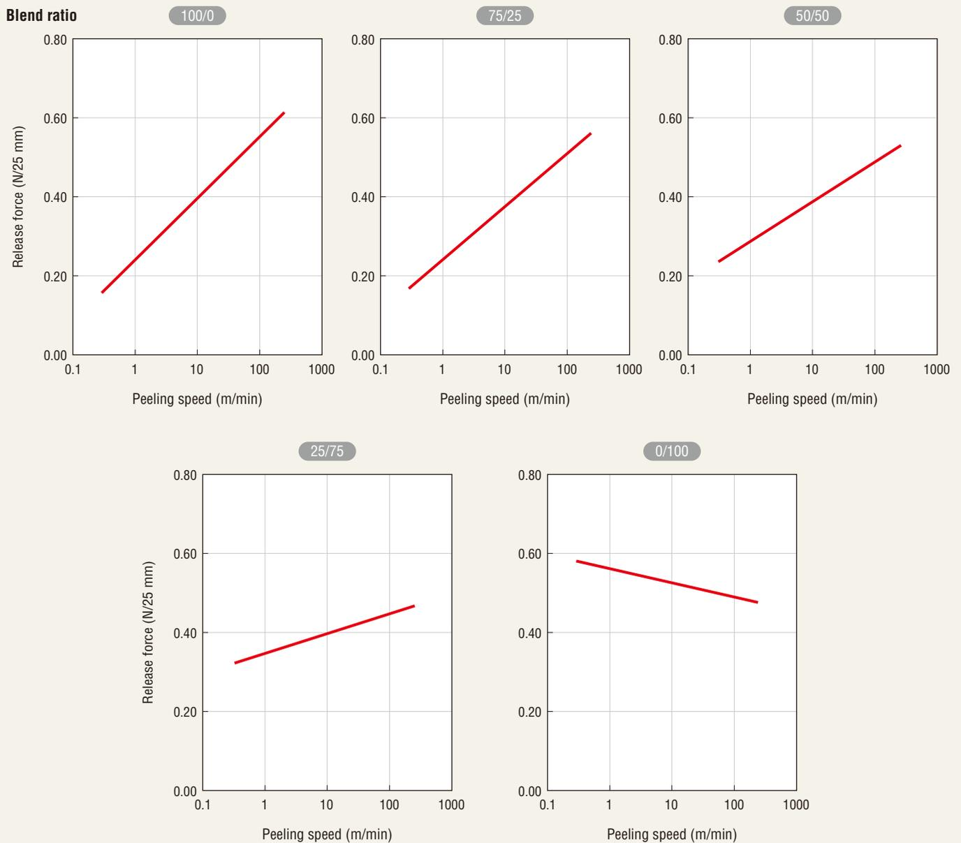
Blend ratio: KNS-330/KNS-340/KNS-338/KNS-347/CAT-CN = 100-0/0-100/10-0/0-10/2 Substrate: polyethylene-coated kraft paper (PEK)
