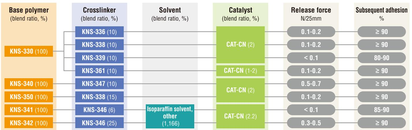
Substrate: polyethylene-coated kraft paper (PEK), Curing conditions: 120 °C×30 sec., Coating weight: 1.1 g/m<sup>2</sup>, Release force test tape: Tesa® 7475
