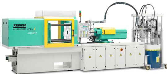
At the epicenter of Lustek’s resources is a 110 ton, All-Electric horizontal liquid injection molding press from Arburg. Additionally, two molds will be utilized—a 4-cavity baby bottle nipple tool complete with cold-runner and valve-gates, and a single-cavity tool designed to overmold silicone onto thermoplastic inserts utilizing SESA’s unique, primerless Selective Self-Adhesive LIMS.
